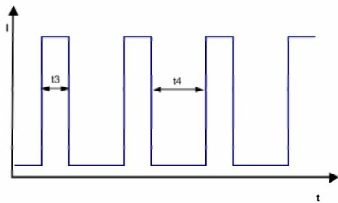
**Locked Rotor Protection:** Locked Rotor protection by cyclical shut down of the output stage.
