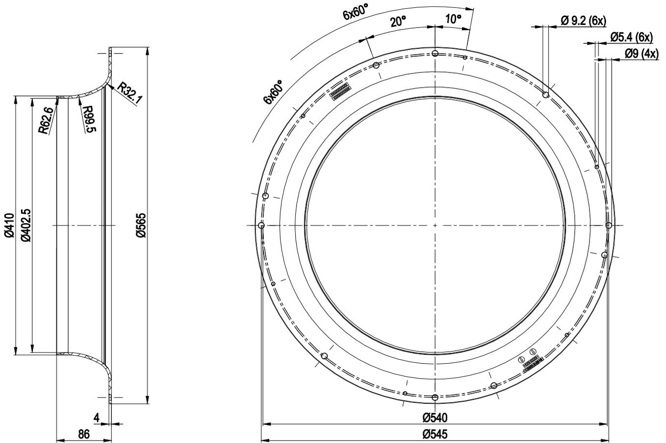
Inlet ring 56902-2-2943 ,tightening torque 5.5±0.8Nm for M5 screw
