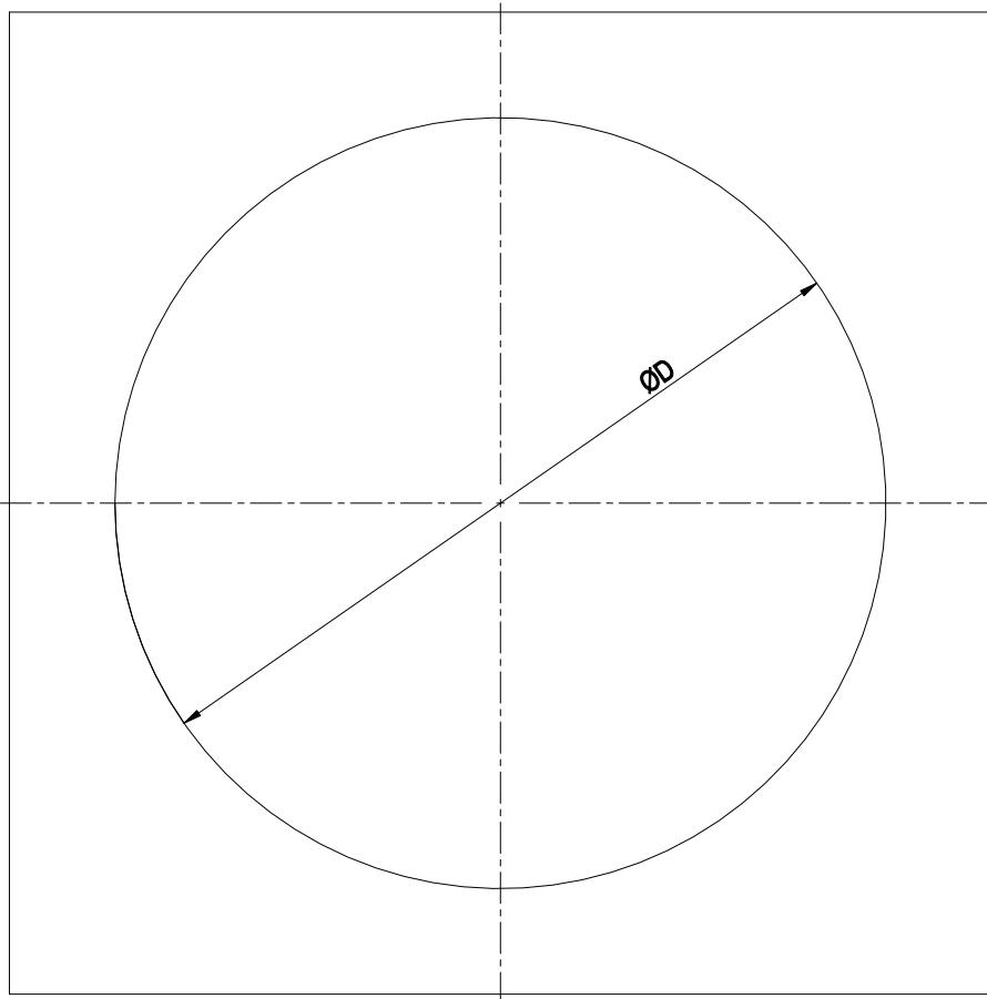
Diameter of the necessary recess for mounting the wall ring in the end device
