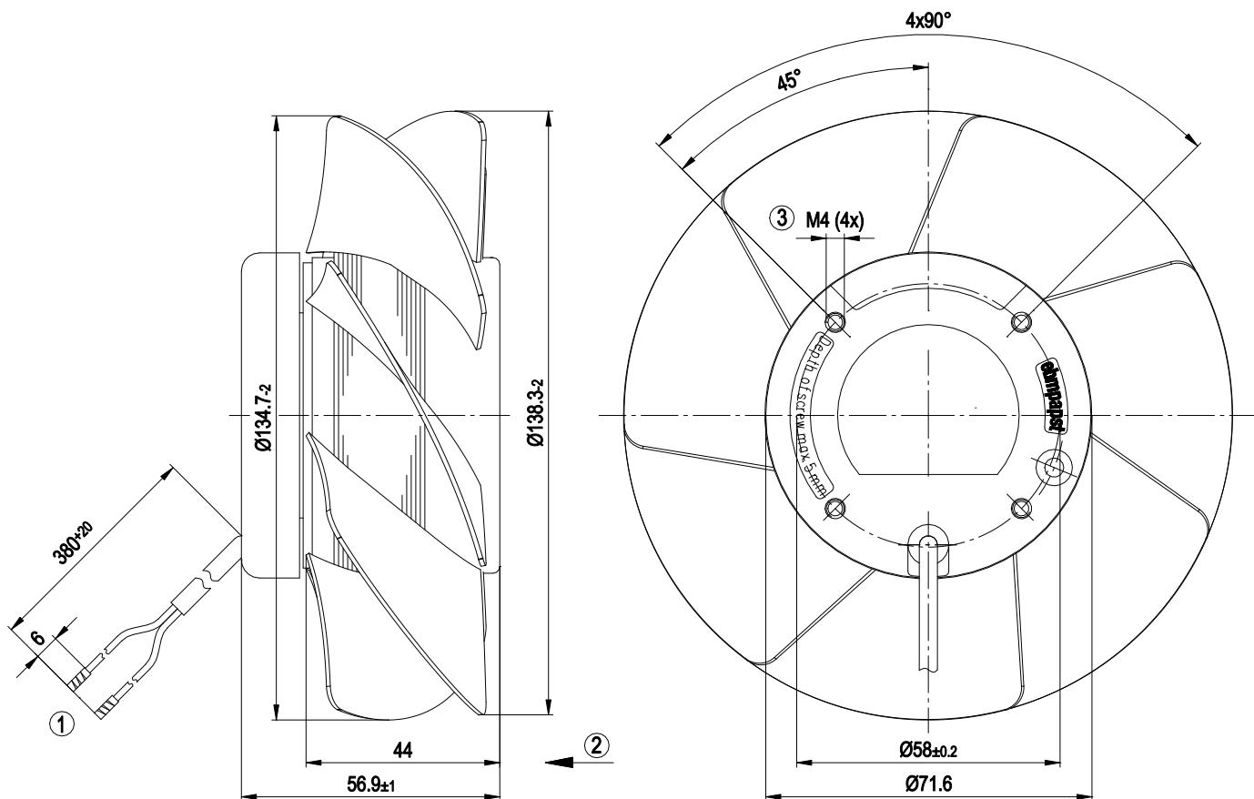
1 Cable AWG20, 2x crimped splices
