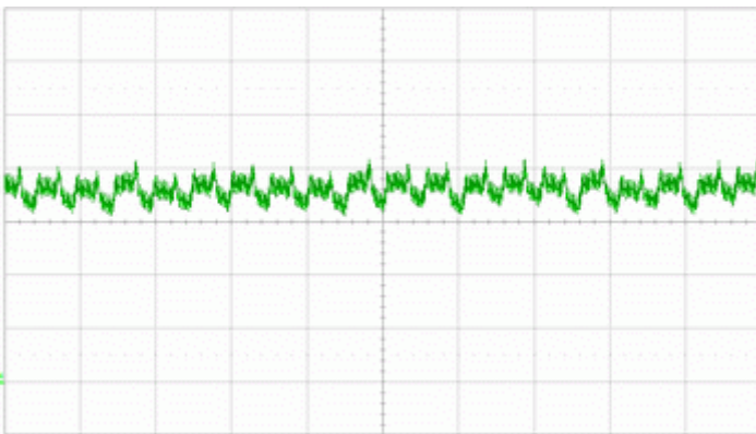
Typical running current at 24 V; 0,5A/div; 2ms/div
