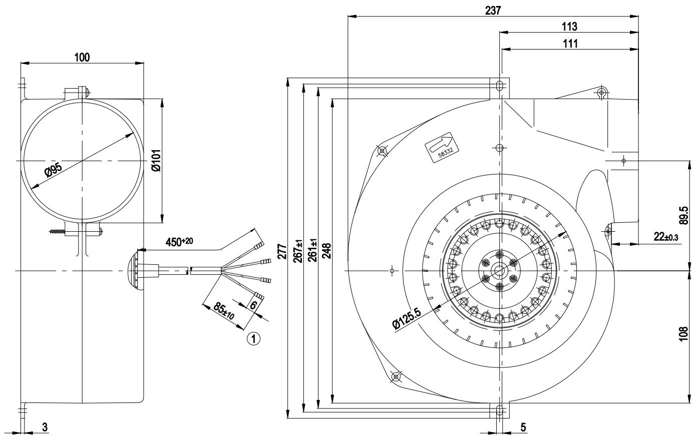
1 Connection line PVC 4 x 0.5 mm<sup>2</sup>; 4 x brass lead tips crimped
