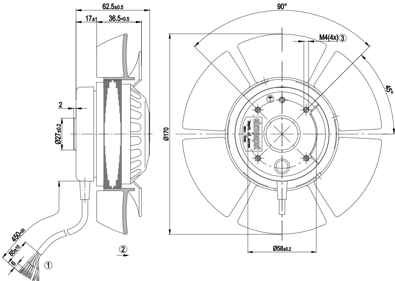
1 Connection line PVC 7G 0.5 mm<sup>2</sup>, 7x brass lead tips crimped
