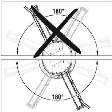
Fig. 3: Cable routing for fans installed upright.
