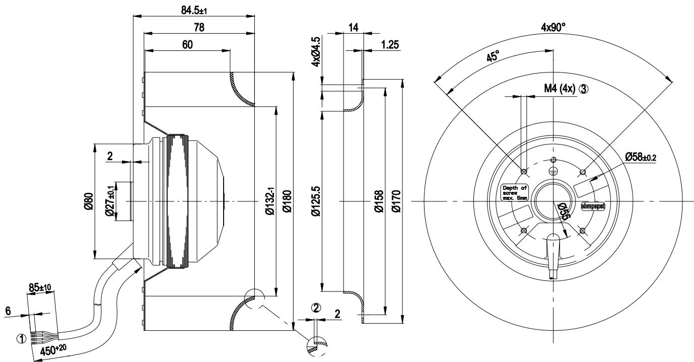
1 Connection line PVC 4 x 0.5 mm<sup>2</sup>; 4 x brass lead tips crimped
