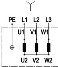
Change of rotation direction by reversing two phases
